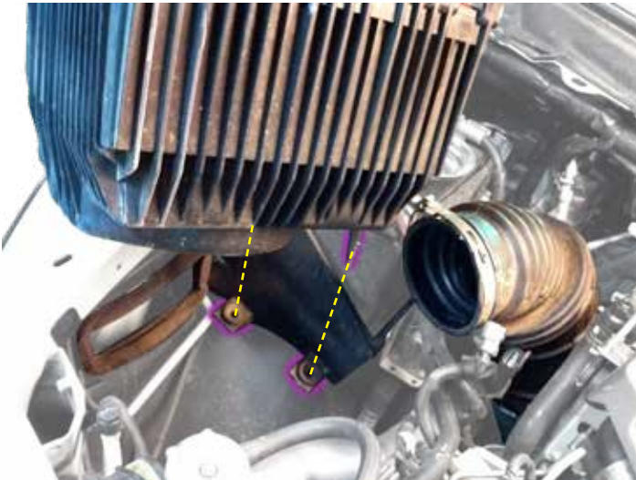
The factory air box has 2 tapered pins that plug into the two grommets shown.
