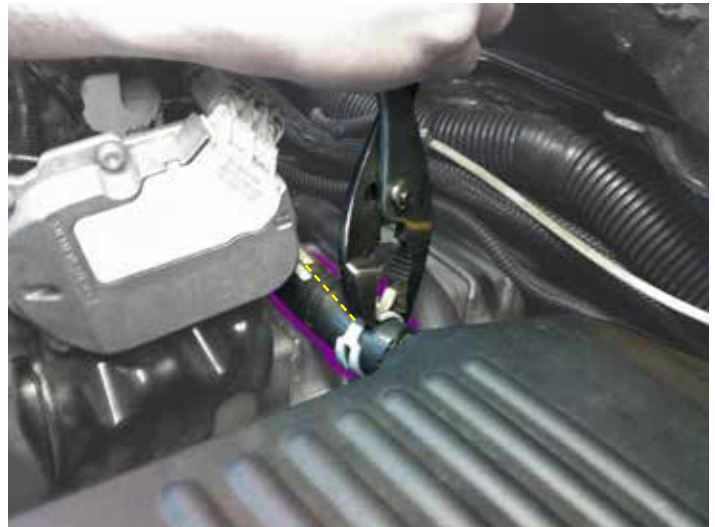
Disconnect the crankcase vent tube from the valve cover by moving the spring clamp shown off the barb on the valve cover.
