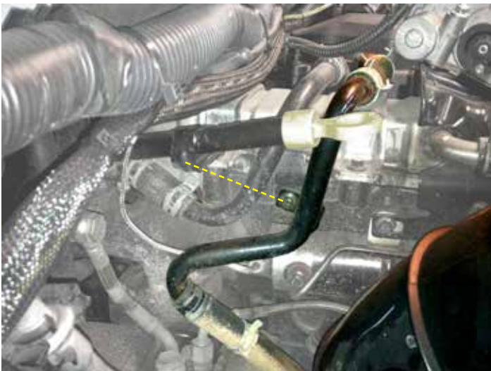
Remove the bolt holding the crankcase breather tube to the block.
