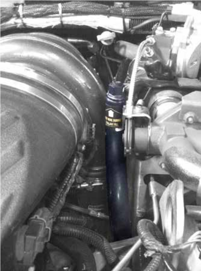
Early EGR System with Solid Tube
